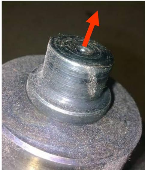
As clutch wear takes place, this button, along with the whole clutch stack assembly, moves in direction of arrow.
