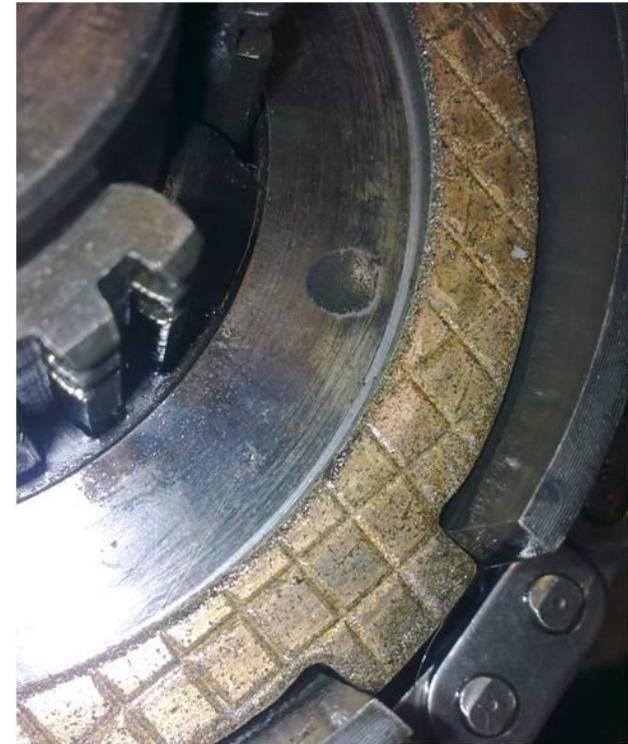
Plate fitted showing relieved area after machining operation has been completed.
