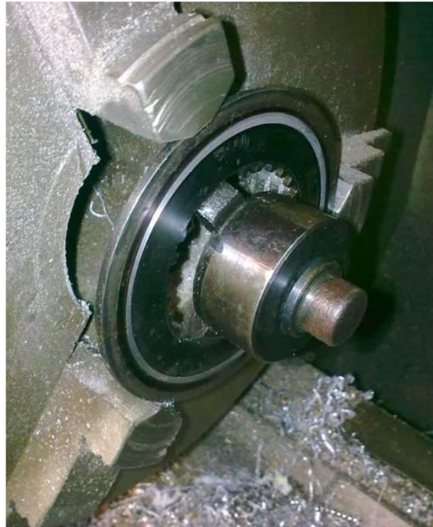
Wear radius removed to provide flat contact face for friction plate. Black line is marker pen.
