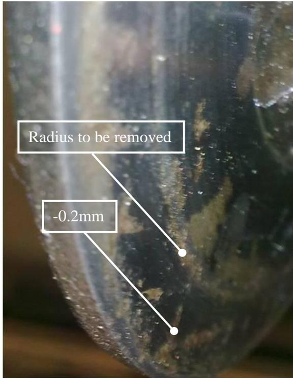
Clutch drum face showing 0.2mm step worn where first friction plate has been driving.
