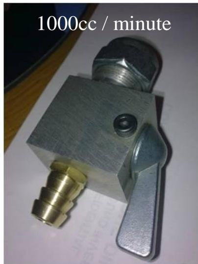
This tap body was made to suit the internals from a Hi-Level 8mm inline tap. The aluminium threaded boss, (M16 x 1 Left Hand Thread) is connected to the main body by using an HTS2000 alloy, or similar, and a simple propane torch with a pinpoint nozzle.
