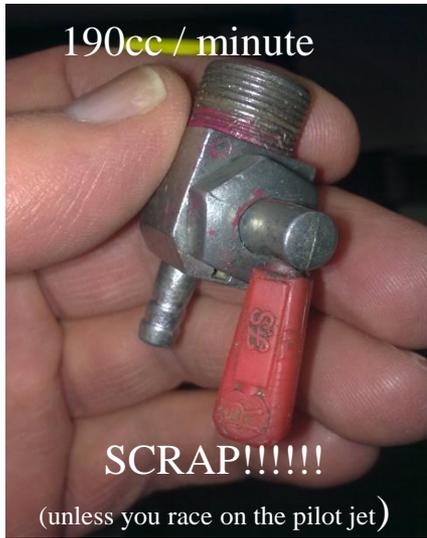
This is the culprit. Don't be fooled that the size of the hole in the outlet tube is governing the flow rate. The ducts going through the rubber valve inside are actually smaller than the outlet bore, so they are the most restrictive part. These are selling on eBay as a Maico fuel tap!
