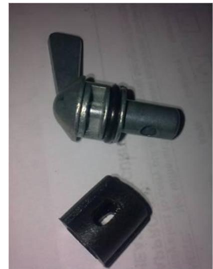
Here are the internals from the Hi Level tap. Rather than dump the main body from the tap, if you clean off the paint and saw it up into pellets, you can use these as the filler to connect the aluminium threaded boss to the billet body, by using a propane torch and the same technique as you would for Lumiweld, HTS2000 or similar.
