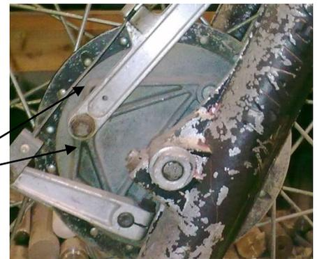
On later models with the standard left mounted brake, the anchor arm is 237mm long between centres, 7mm longer than the right mounted anchor arm. This also helps bring the web more into line with the anchor arm by about  $5^\circ$
