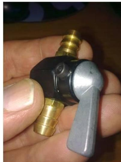
The only suitable taps I could find where they were quoting a good flow rate were about \$100 dollars each. I needed one plus a spare, so I decided to go for the Hi Level option and mill the bodies from billet. You can buy these Hi Level taps for about £8.
